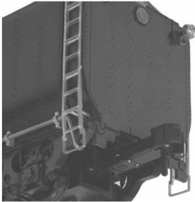
Figure: MTH ProtoCoupler in higher position.
