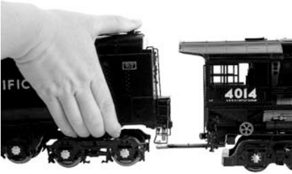
Figure: Connecting Locomotive to Tender
